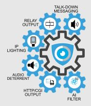
CHeKT's Automation Rules allow security companies to utilize camera analytics to create a proactive alarm response. CHeKT will automatically initiate audible and visual responses using IP Speakers and relays when an alarm occurs from any of these systems.
