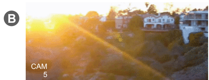
CCTV Image Affected by Sunlight
